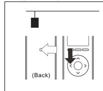
1. Press the [RESET] on the back of transmitter + [IP1] button. The motor shaft will rotate back and forth shortly to indicate that it is in adjusting mode for Limit 2.
