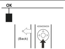
3. Press [RESET] on the back of transmitter + [BACK] button, the motor will quiver for a moment and the process will be finished.
