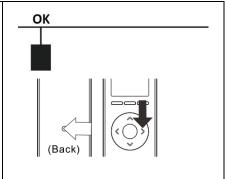
3. Press [RESET] on the back of transmitter + [IP2] button, the motor will quiver for a moment and the process will be finished.
