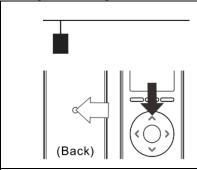
1. Press the [RESET] on the back of transmitter + [GO] button. The motor shaft will rotate back and forth shortly to indicate that it is in adjusting mode for Limit 1.
