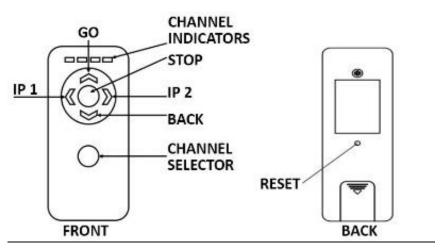
Before using the remote control functions, user must pair the remote to the motor.
