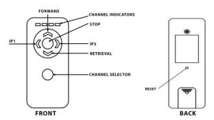
Before using the remote control functions, user must pair the remote to the motor.
